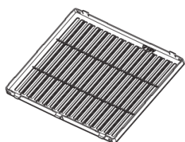
Inlet frame Washable pre-filter
